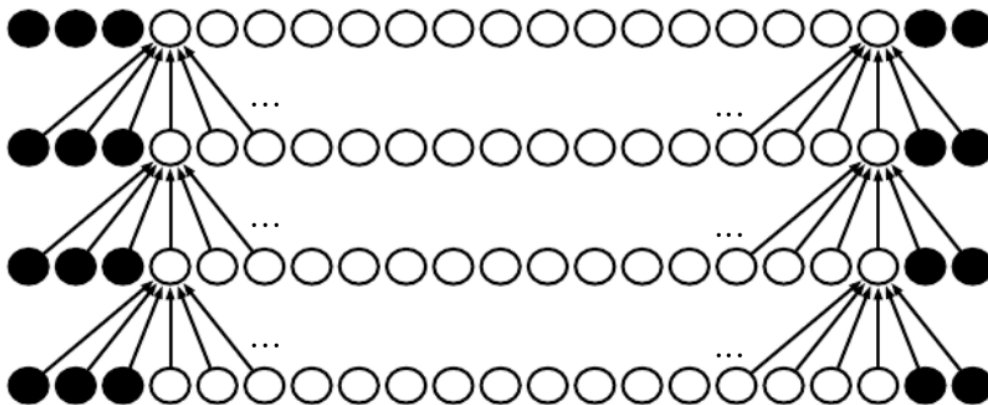
Figure 2.14: The effect of convolution with same padding on output size [7]
