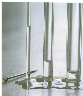
Figure 2.1. Vertical pipes with different diameters. Heights and shape of the meniscus are different.
